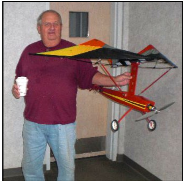
Paul Meier (above) with his GYLO plane, scratch built with an electric motor using a 3000 mah battery. The wings are similar to paraglide “wings.”
