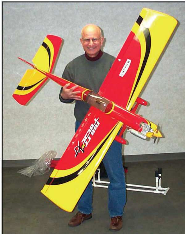
Jam Rabii showed a Pulse XT 60 with a wing span of 70", weight 6-7 pounds. It has an OS-61 engine and a Spektrum 6200 receiver.
