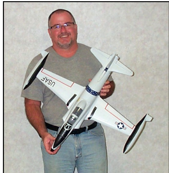
Richard Bombardier shows his Sky Angel T-33 55mm EDF foam aircraft, from Banana Hobby. It has a 30" wing span, a 20 amp ESC and a Spektrum 2.4 GHz radio. It weighs 13 ounces.
