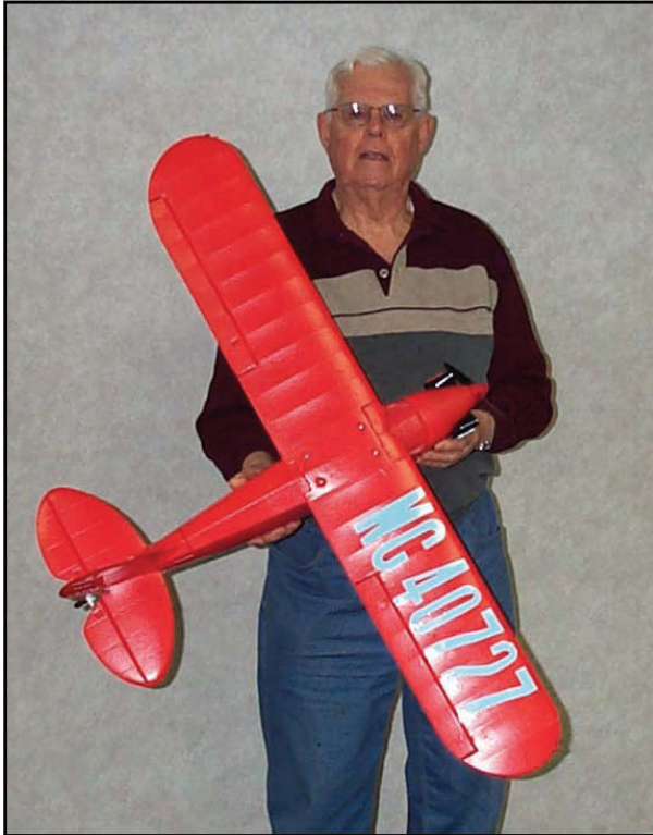
Hob Davis shows his Piper J-5 from Hobby Lobby. It has an outrunner electric motor with a Spektrum radio powered by a 2-cell lipo 1600 mAh battery.
