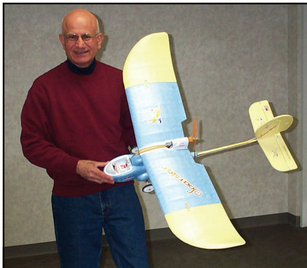
Jam Rabii shows this Soarstar foam trainer with a 300 size electric motor. It has a Spektrum radio and a 1250 mAh battery.
