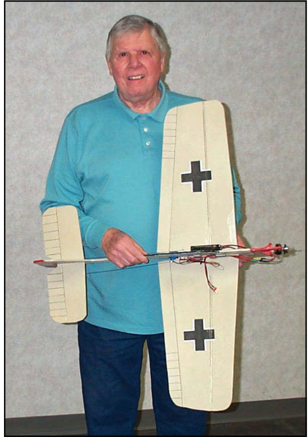
This foam Focke wulf belongs to Bill Fishbach. It has a 35" wing span, a Spektrum radio 3 channel, with a 1300 mAh battery driving a 300 motor.
